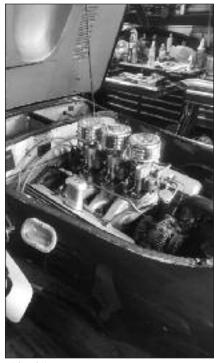
Mr. DiCola has been feeling fairly energetic of late and has been taking it out on the editorial Allard J2. He has rebuilt the engine, replumbed the fuel system, and replaced the fuel cell ( we put the first one in only about twenty years ago... apparently they just don't last...) Additionally the lights are being rewired and the brakes have gotten some attention. Mechanically the old girl should be as good as she was when we first rebuilt her.
